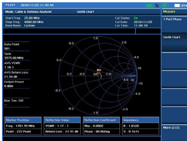
Cable and antenna test — Smith Chart
