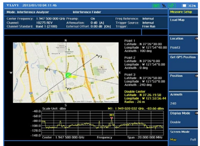
Interference analysis test — Interference Finder
