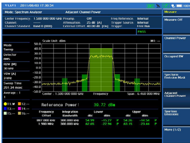
RF test — Adjacent Channel Power
