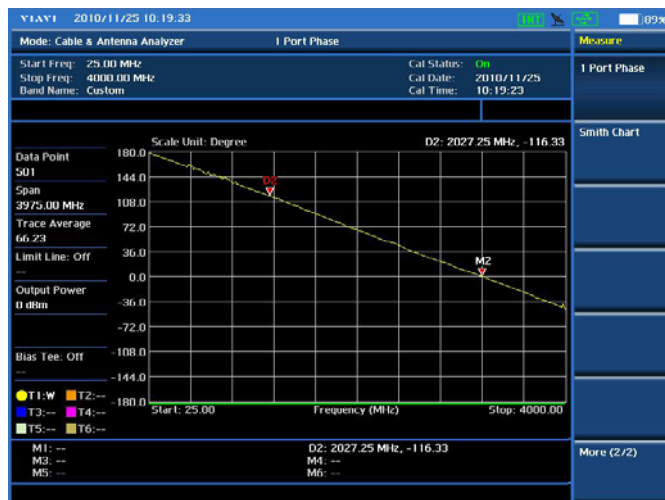
Cable and antenna test — 1-Port Phase
