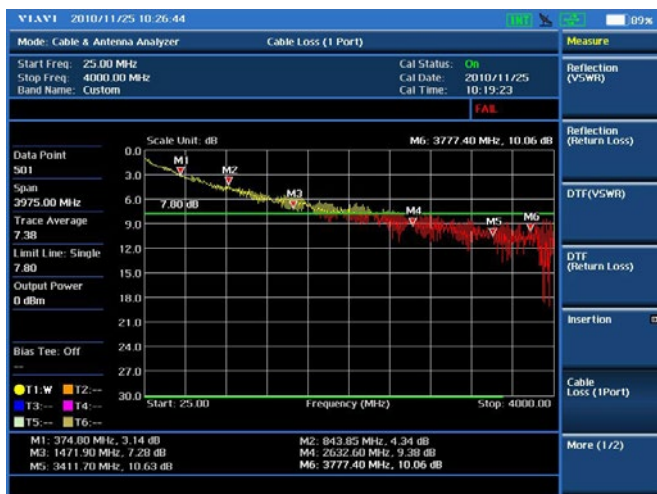
Cable and antenna test — Cable Loss
