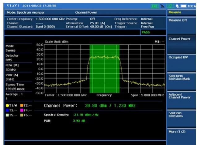
RF test — Channel Power
