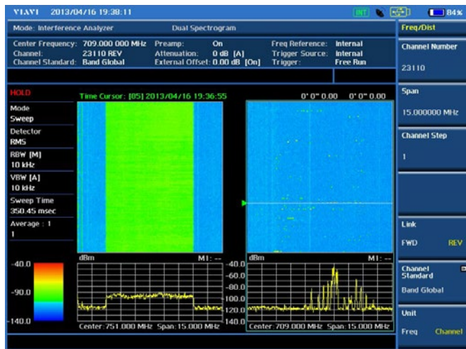
Interference analysis test — Dual Spectrogram
