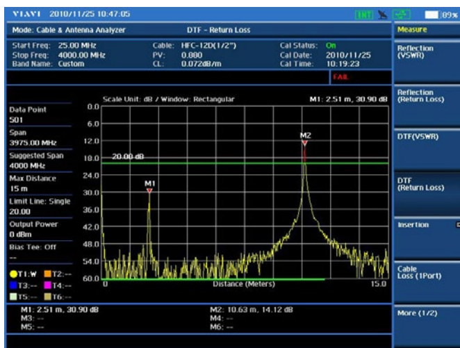
Cable and antenna test — Distance to Fault
